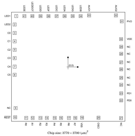
\* The IC substrate should be connected to VSS in the PCB layout artwork.
